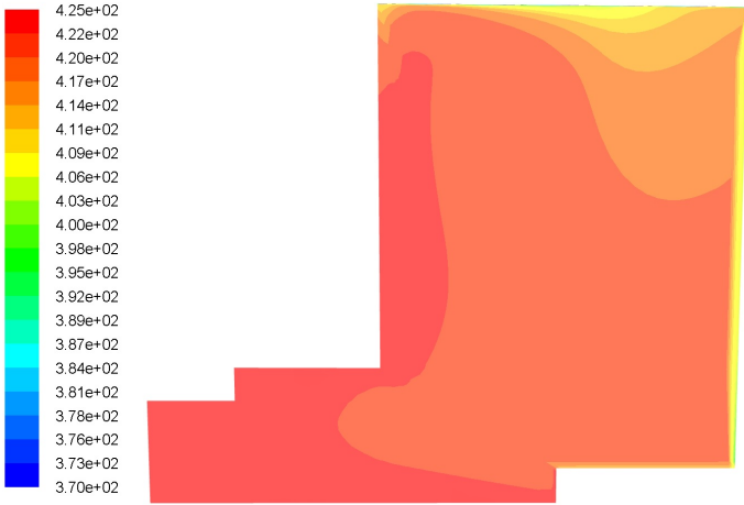
FIGURE 9: OIL TEMPERATURE CONTOURS (K) IN THE BEARING CHAMBER FOR ANGLE CUT \theta = 15^\circ
