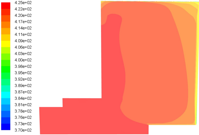
FIGURE 8: AIR TEMPERATURE CONTOURS (K) IN THE BEARING CHAMBER FOR ANGLE CUT \theta = 15^\circ
