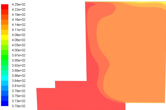
FIGURE 10: MIXTURE TEMPERATURE CONTOURS (K) IN THE BEARING CHAMBER FOR ANGLE CUT \theta = 15^\circ
