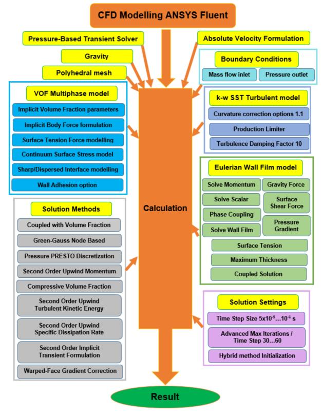
AMBEC's methodology for CFD modelling of thermal and hydraulic processes in the aircraft engine bearing chamber
